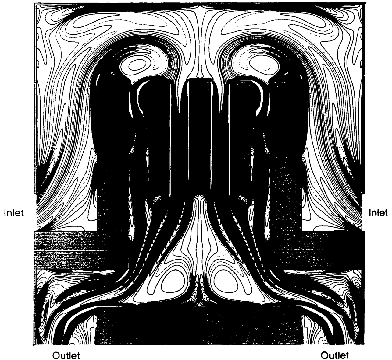
Figure 5.7: Vorticity plot with 30 equally spaced contours from 1 to 100 and from -100 to -1, at time t_3 = 1.5 , of the flow past the cooling system. Re = 2000 . The computation is based on EC4 method with the resolution \Delta x = \Delta y = \frac{1}{512} .
